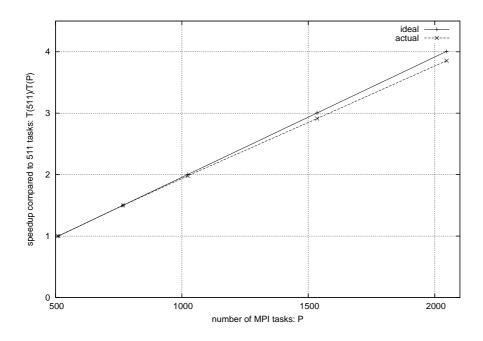
Figure 15: Speedup for model with 4 million cells and 2 billion synapses simulated with SPLIT on BG/L (from Djurfeldt et al., 2005).
