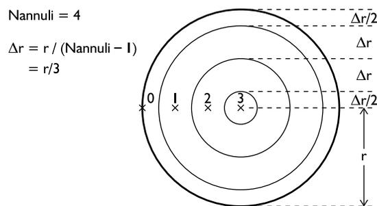
Figure 9.9. Diagram of the concentric shells used to model radial diffusion. The × mark the radial distances at which concentration will be second order correct in space.
