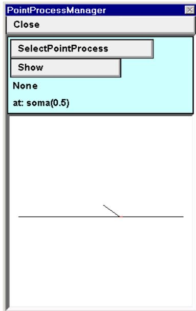
A. Note the labels in the top panel. None means that a signal source has not yet been created. The bottom panel shows a stick figure of our model cell.
