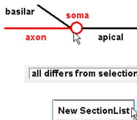
With the **Select One** radio button on (Fig. 1.14), click on the axon and soma sections while holding down the shift key. The selected sections will be indicated in red . . .
