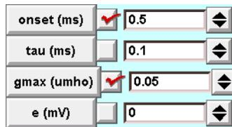
D. For this example change onset to 0.5 ms and gmax to 0.05  $\mu$ S; leave tau and e unchanged.
