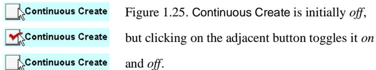
If we make any changes to the model while Continuous Create is *on*, the CellBuilder will automatically send new code to the interpreter. This can be very convenient during model development, since it allows us to quickly examine the effects of any change. Automatic updates might bog things down if we were dealing with a large model on a slow machine. In such a case, we could just turn Continuous Create *off*, make whatever changes were necessary, and then cycle it *on* and *off* again.
