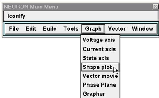
A. The first step is to create a Shape plot by clicking on Graph / Shape plot in the NEURON Main Menu.
