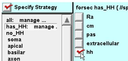
Select the has\_HH subset in the middle panel, and then toggle HH *on*.
