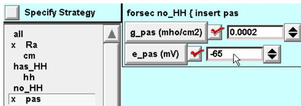
The final values of g\_pas and e\_pas. Not shown: cm (all subset) and the parameters of the hh mechanism (has\_HH subset), which have the desired values by default and do not need to be changed, although it is good practice to review them.
