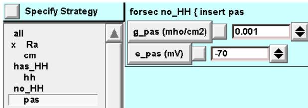
The sections in the no\_HH subset have a passive current whose parameters must be changed from their defaults (shown here).
