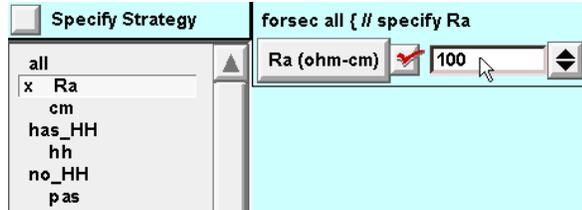
For the subset all, change the value of Ra from its default (80  $\Omega$  cm) to the desired value of 100  $\Omega$  cm.
