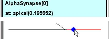
C. Clicking on a different point in the shape plot moves the synapse to a new location. This change is reflected in the top and bottom panels of the PointProcessManager.
