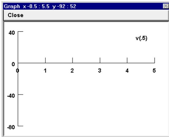
B. In the graph that appears, the horizontal axis is in milliseconds and the vertical axis is in millivolts. The label  $v(5)$  signifies that this graph will show  $V_m$  at the middle of the default section. With the CellBuilder, this is always the root section, which in this example is the soma (the concepts of "root section" and "default section" are discussed in **Chapter 5**).
