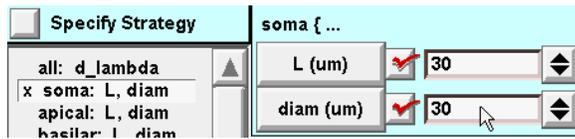
After doing the same for diam, the dimensions of soma should look like this. The checkboxes adjacent to the L and diam buttons indicate that these parameters have been changed from their default values. The x in the middle panel is another reminder that at least one of the parameters associated with soma has been changed.
