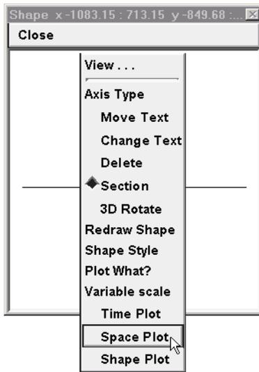
C. Right click in the Shape plot window to bring up its primary menu. While still pressing the mouse button, scroll down the menu to the Space Plot item, then release the button.
