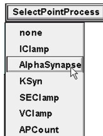
B. SelectPointProcess / AlphaSynapse creates a point process that emulates a synapse with a conductance change governed by Eq. 1.1, and shows us a panel for adjusting its parameters.
