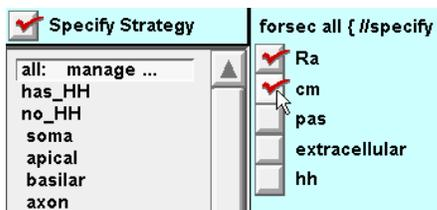
For the all subset, toggle Ra (cytoplasmic resistivity) and cm (specific membrane capacitance) *on*.
