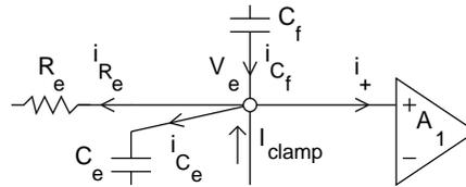
Fig. 3.8. The third node of the circuit in Fig. 3.6. Perfect compensation for electrode capacitance (which can never be achieved with real amplifiers and electrodes) requires that  $i_{C_f}$  balances  $i_{C_e}$  exactly.
