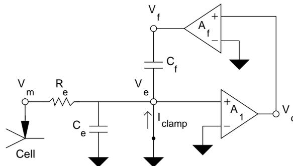
Fig. 3.6. Capacitance compensation under current clamp. The capacitance  $C_e$  of the microelectrode distorts recordings by slowing and attenuating the response of  $V_e$  to changes in  $V_m$  and  $I_{\text{clamp}}$ . Amplifier  $A_f$  and capacitor  $C_f$  compensate for this by supplying charging current to  $C_e$ .
